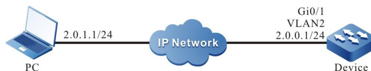
Figure 5 Network Topology for Configuring a Local Terminal to Telnet to the Device
