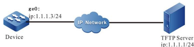
Figure 27 Networking for configuring bootloader to start the image program via the network
