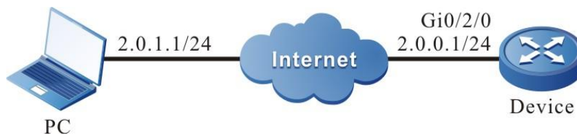
Figure 12 Configure the local device to log into the remote device via web
